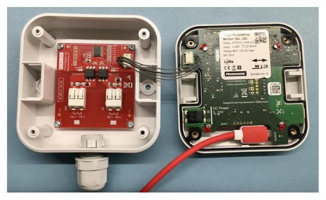
Connect the sensor to your Computer using a USB Cable.
