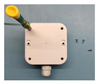
Remove the four screws from the casing to gain access to the device.
