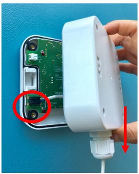
Before closing the casing, make sure that the two components are aligned as depicted:
