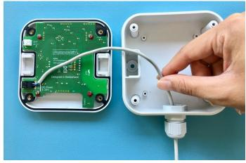
Guide the cable through the cable gland.
