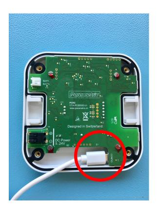
Connect the sensor to your Computer using a USB Cable.
