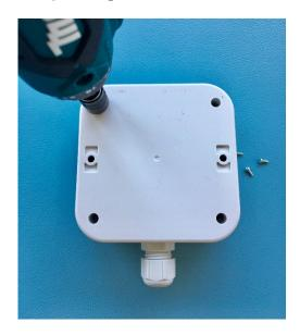
Remove the four screws from the casing to gain access to the device.
