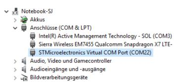
After connecting the PCR2 to your PC, you should see a new device appearing in Windows Device Manager.
